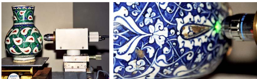
Figure 1: The Raman analysis of a glazed ceramic. The choice of the right microscope objective enables selective examination of the over- and underglaze décor as well as the slip or glaze-body interphase. The photographs show on-site analysis of Iznik artefacts performed at the Musée national de Céramique, Sèvres, using a remote fibre optic probing through laser/spectrograph coupled microscope objectives (magnification x800); note the 3D micrometer support below the optical head. Also, the effective laser spot is much smaller than its visible halo. (Photographs © Ph. Colombar)
